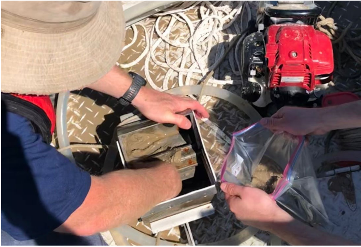
Figure 2.10: Example of sediment documentation and sampling from onboard survey vessel
