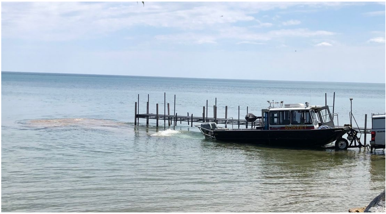
Figure 2.8: Prop Wash Exhibited During Vessel Takeout
